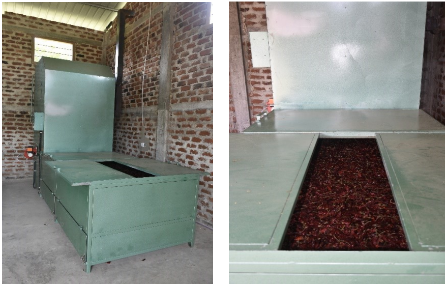
Figure 4.3: Chili Dryer Provided by the Agriculture Sector Modernization Project
